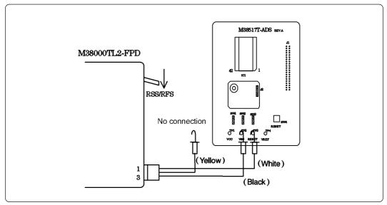
Figure 4.3 Connecting the M38517RSS
